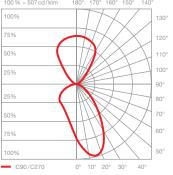
wide light beam (up and down), beam angle approx. 80° directed (down)
