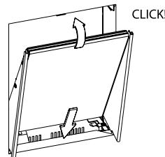
insert the reflector, underside first.
