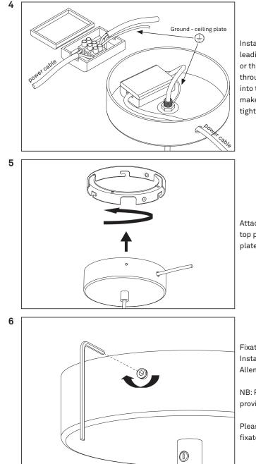
Install the power cable by leading it through either the top or the side of the ceiling plate through the cable relief and into the cable connector. Please make sure the cable relief is tightened.
