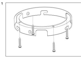
Mount the top plate to the ceiling with screws.
