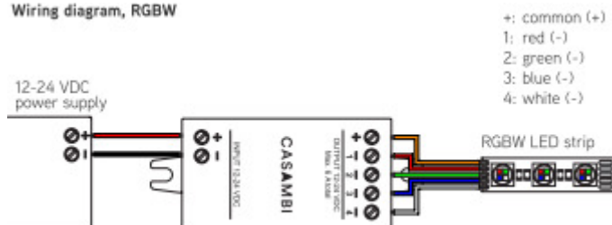
Wiring diagram, RGBW
